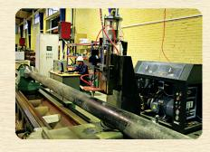
The slotting machine (Abrasive WaterJet) is custom designed, as this process is unique to this innovative product. Our facility is now fully operational and many of our major clients have viewed the facility and audited the processes. The expansion tests of SES Screens and all related tests for SES Hanger Packer have been successfully performed, based on customers' needs.
